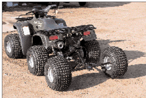
The rear suspension and wheel assembly moves independently of the ATV's suspension. The track was designed to ride on a pair of Carlisle tires.
