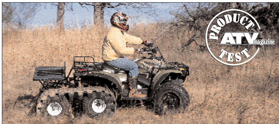
The Tru Trax System dramatically increases flotation. This setup minimizes environmental impact on soft soils.
